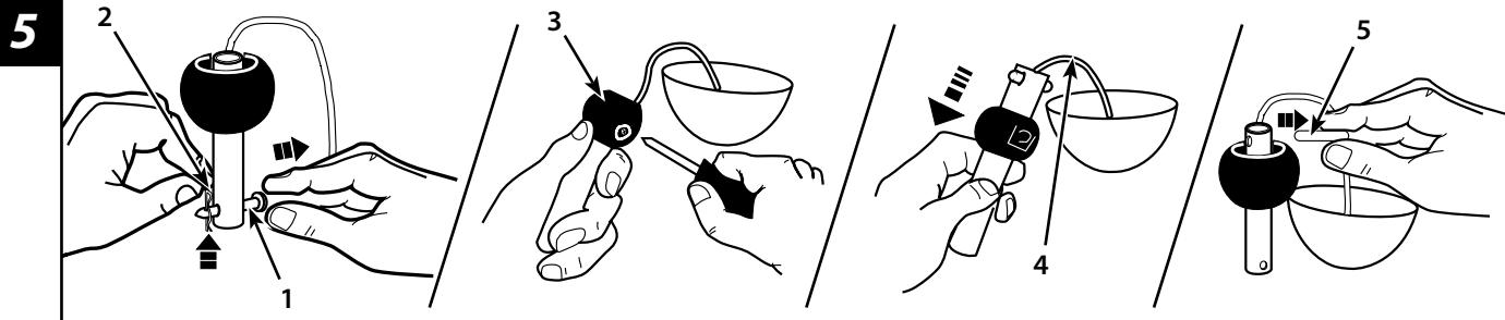
**GB** Remove clamp pin (2) and cross pin (1) from downrod. Loosen setscrew in downrod ball (3) until ball moves easily up and down the downrod. Do not remove ground wire (4) from downrod ball. Slide downrod ball down, exposing cross pin (5). Do not remove ball completely. Remove cross pin and save for later use.
